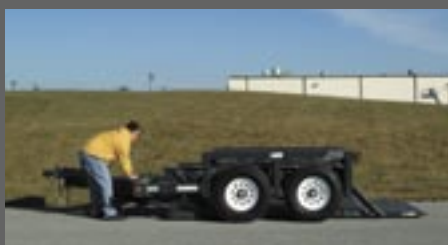
Lower entire deck to ground level
