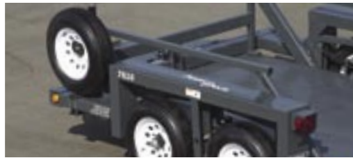
Spare Tire & Bracket Mounts conveniently within the width of the chassis.
