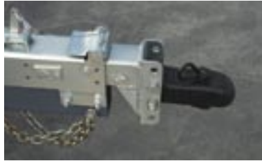
Surge Brakes Heavy-duty actuator with adjustable coupler.
